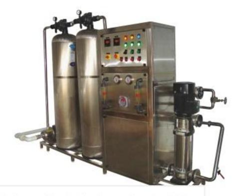
All the Control devices are fitted inside the control panel, which is mounted on the machine itself. All the motors have thermal relays which protect them against voltage surges and excessive current.
